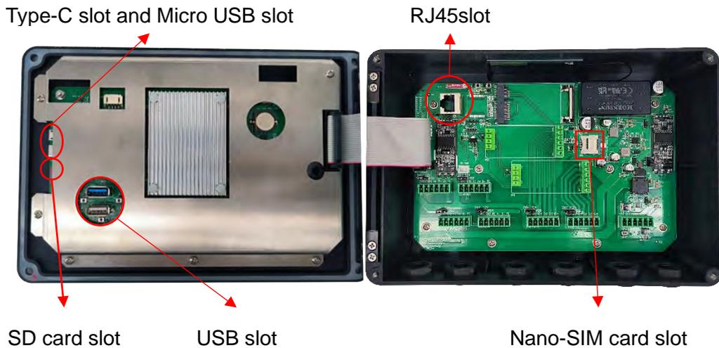
MC-W-S is equipped with Nano-SIM card slot and SD card slot. Insert the Nano-SIM card, the MC-W-S will automatically connect to the network and upload the data to the cloud platform. By default, the company's cloud platform is uploaded. To switch other data platforms, please check the configuration information. MC-W-S comes standard with a 32 GB SD card.
