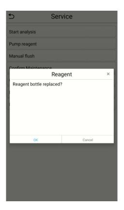
Clicking on [**Pump reagent**] will pump the reagent for 60 s. After canceling or pumping the reagent, you will be prompted, [Reagent bottle replaced?] Click [**OK**] and the reagent level will be reset.
