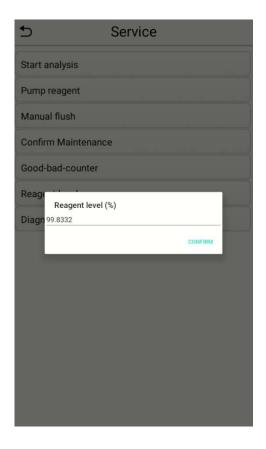
Click on "Reagent level" to view the reagent level and set the percentage of reagent level.
