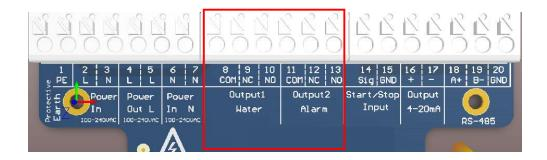
The relays are designed as change-over contacts, with a common connection and the switching outputs NC and NO.
