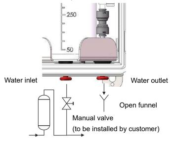
The inlet pressure of the water sample must be between 0.5 and 5.0 bar.
