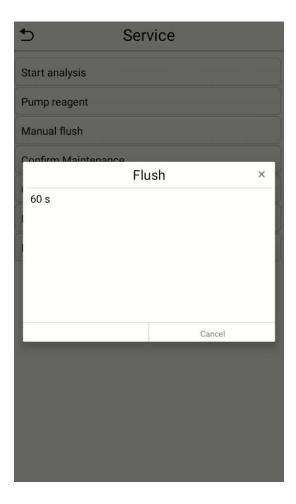
Clicking [Manual flush] will open the unit's solenoid valve and the water sample will flush the unit for 60 seconds.
