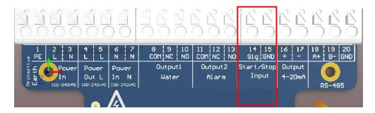
Start/Stop Input: Start input contact for analysis / flow switch / Interval reset
